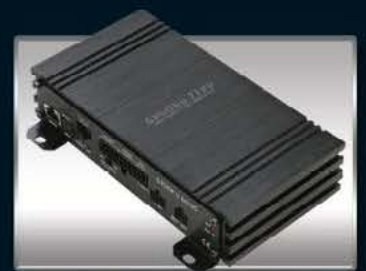
GZDSP 4.60ISO (4x40w) Plug & Play 4 Channel Amplifier with integrated DSP
